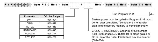
Any Caller ID circuit can be assigned to any analog ground or loop start CO line circuit. Circuit numbers do not have to match.
