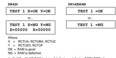
An X=NG or Y=NG RAM test result indicates a defective RCTU PCB; change the appropriate (X or Y) RCTU PCB and retest RAM on the newly installed RCTU.
