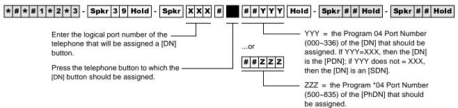
Directory Numbers are assigned to the flexible button positions on telephones.
