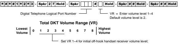
Set VR 1~4 for initial off-hook handset receiver volume level VR resets to programmed level (1~4) after each call (onhook/off-hook). Each level is equivalent to a 2dB change.
